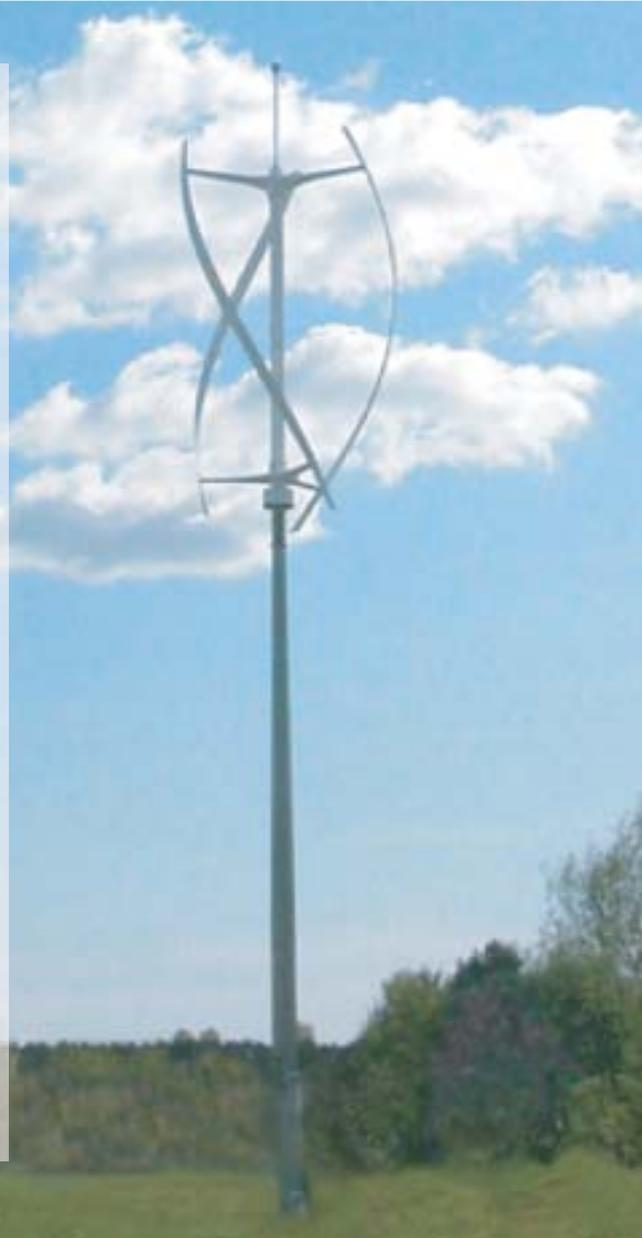
The QR5 turbine costs £25,000 including generator, anemometer, accelerometer and peak power tracking hardware. Additional costs include control electronics, mast and mounting, and mechanical installation. Total costs typically range from £30,000-£35000 per installed turbine. The QR5 has a design life of 25 years and comes with a two year warranty.
